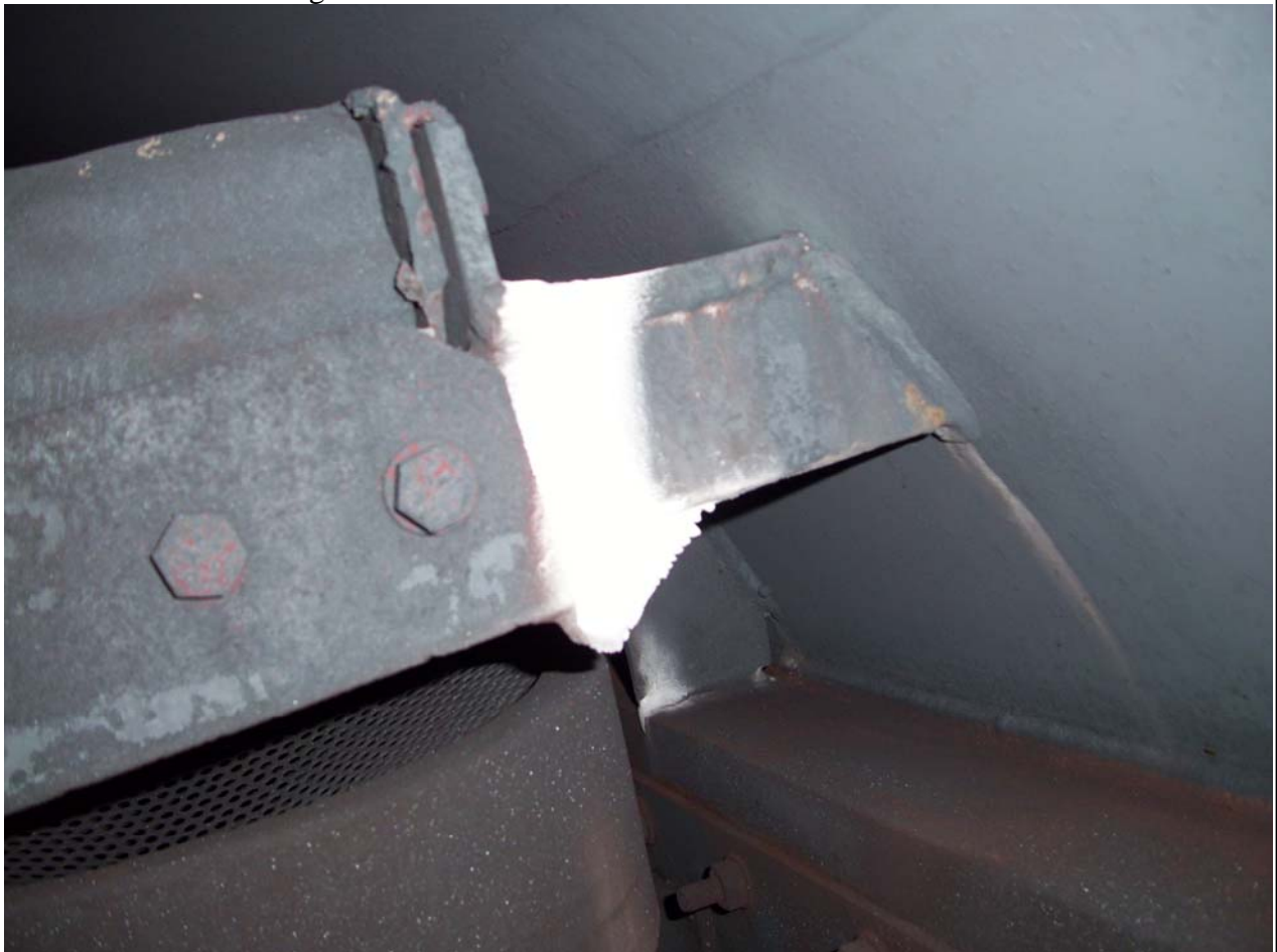
Photo 2: The drum is with the mark of excess of phosphate in the drier area.
